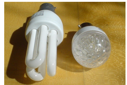
Figure 9.4. Philips 11 W alongside Omicron 1.3 W LED bulb.
