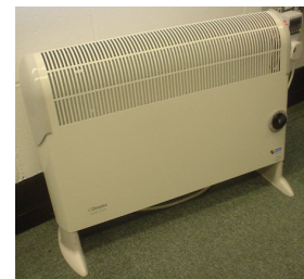
Figure 7.6. A big electric heater: 2 kW.
